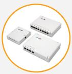
The Capsule Axon series is a highly reliable, serial-to-network bridge designed to connect up to x8 serial medical devices such as patient monitors, ventilators, pumps to the to the hospital network. Once data is managed by the Capsule server, it can be integrated to clinical documentation systems to aid in accurate charting or other clinical applications.
